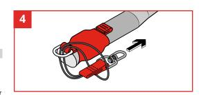
Apply Swivel Catch by choking through the D-Ring in the Tool Catch.
