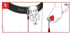
Your hammer is now ready to be applied to a GRIPPS® tether. Always consider the max load of your tool holster, in conjunction to weight of the hammer.
