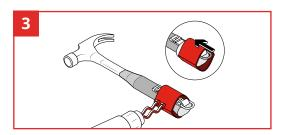
Slide Gripp Shrink over Tool Catch and V-Gripp Tape. Then apply heat gun.
