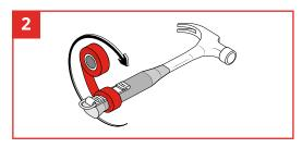
Wrap the tape around the tool while stretching the tape to activate the self-vulcanizing feature, creating a secure connection. Ensure raised 'catch' is not covered by the tape. Pull on Tool Catch with force to test application.
