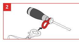
Apply the GRIPPLink to the tool shaft. Where possible, insert tool through the smallest end of Gripplink.
