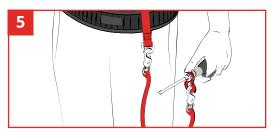
Connect a tether up to 25cm in length to the GrippLink.
