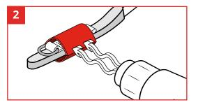
Apply a heat gun to the Gripp Shrink. This will cause Gripp Shrink to shrink in size and adhere to your Tool Catch/V-Gripp Tape. Use heat gun evenly and rotate tool continually whilst applying heat. Allow to cool
