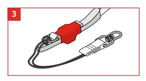
The D-Ring of your Tool Catch is now ready to be connected with a suitable GRIPPS tether or Swivel Catch.
