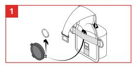
Remove Tool Ring from retractor then insert the Retractor Unit into back pouch, then reattach tool ring.
