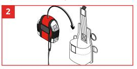
Attach Swivel Catch to the Retractor Unit D-Ring. Slide holster onto work belt and situate on belt as desired.
