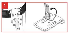
To connect to a work belt, thread work belt through the loop on back of holster. Open holster by unclipping button.
