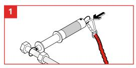
Attach a suitable GRIPPS tether to the small wire loop at base of Bolt Gripper.
