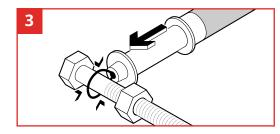
Slide the wire noose over your bolt/nut and slide up till reaching the top of your screw is reached. Release the shaft to secure tightly.
