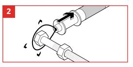
Compact the Bolt Gripper shaft downwards by firmly pressing with your fingers on the shaft, this will expand the opening.
