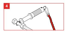
Once securely tightened. You can proceed to work with your bolt as required. Repeat process in reverse to remove.
