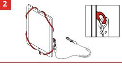
Attach Coil Tether to one of the two eyelets. Connect opposite end of tether to an appropriate anchor point.
