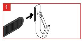
To connect to a work belt, thread work belt through the loop of Battery Operated Arrest Holster. Slide Belt-Loop Anchor along the work belt to where you want it positioned.
