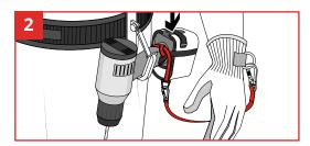
Your tethered drill (or similar device) can be stowed into the BOA after by simply pressing your tool into the latch. The latch utilizes a spring to automatically lock after. To remove your tool, press latch inwards and pull tool out. Ensure your tool is properly anchored before using BOA holster.
