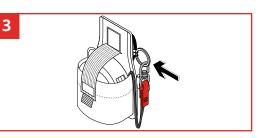
Tether your tool or GRIPPS® Swivel Catch directly to the retractor unit tool ring.
