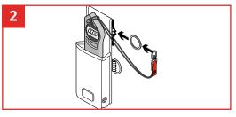
Thread tool ring back onto Retractor. The tool ring should be exposed outside of the holster.
