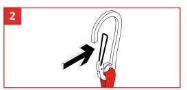
To attach Single-action style carabiners (H1062 or H01068) to a tool connector, push tool connector into the carabiner until it clicks shut.
