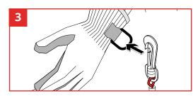
Example application with H01062 attaching to a glove anchor point.
