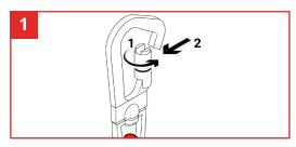
To attach a carabiner to a tool connector with H01069, twist the carabiner lock in a counter-clockwise direction to unlock.
