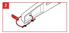
Join the two ends together, ensuring a firm application and click sound is heard/felt. Test Gripplock Cable cannot be separated by tugging both ends firmly.
