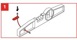
Feed the Gripplock Cable through the pre-formed hole in the tool.
