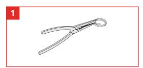
Pry the two halves of Tool Ring open with a set of ring pliers or needle nose pliers.
