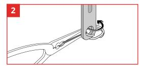
Using the needle nose pliers, thread the pried-open halves of the Tool Ring into the tool aperture. Rotate the Tool Ring until both halves of the Tool Ring are inside the tool aperture and the tool is secured.
