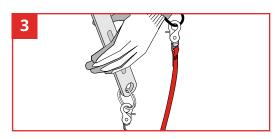
Once the tool ring is applied to your chosen tool, connect the tool ring to a GRIPPS® tether of choice.
