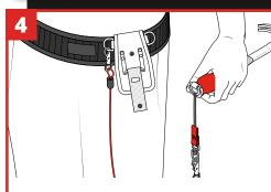
Your hammer is ready to apply to a GRIPPS® tether. Always consider the max load of your tool holster, in conjunction to weight of the hammer.
