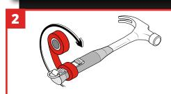
Wrap the tape around the tool 10x while stretching the tape to activate the self-vulcanizing feature, creating a secure connection. Ensure raised 'catch' is not covered by the tape. Pull on Tool Catch with force to test application.
