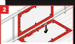
For use on gridmesh flooring, lie Gap Mat flat and apply ties to eyelets.
