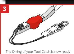
The D-ring of your Tool Catch is now ready to connect with a suitable tether or wwivel catch.
