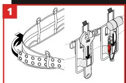
Weave the work belt through the inner side loops of the H01118 back support. At the same time, apply tool holsters to the belt by sliding on each holster (or unbuckle the holster back clip and fold the holster strap over the belt).
