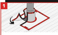
Surround pipe with Gap Wrap. Overlap central Velcro fasteners strips.
