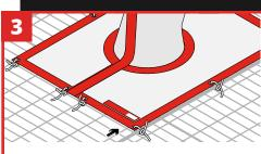
Fasten all outer eyelets to gridmesh with suitable ties. Ensure no excessive amount of ties are exposed that may cause a trip hazard.
