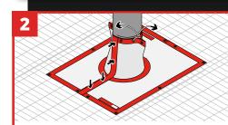
Ensure the fastener strip is firmly pressed all the way along from top to bottom. Fasten all eyelets around piping with suitable ties.
