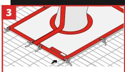
Fasten all outer eyelets to gridmesh with suitable ties. Ensure no excessive amount of ties are exposed that may cause a trip hazard.
