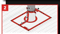
Ensure the fastener strip is firmly pressed all the way along from top to bottom. Fasten all eyelets around piping with suitable ties.
