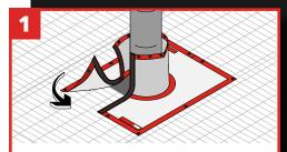
Surround pipe with Gap Wrap. Overlap central Velcro fasteners strips.
