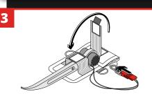
Slide tool into holster with connection point applied to tool.
