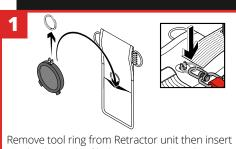
into back pouch of holster. Reattach tool ring, keeping the ring exposed outside holster.
