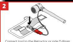
Connect tool to the Retractor or side D-Rings.
