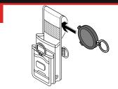
Insert second Retractor Unit into rear pouch. Ensure tool ring is exposed outside holster.
