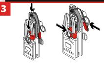
Connect tool to the Retractor or side D-Rings.
