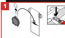
Remove tool ring from Retractor unit then insert into back pouch of holster. Reattach tool ring, keeping the ring exposed outside the front of the holster.
