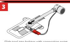
Slide tool into holster with connection point applied to tool.
