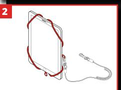
Attach a tether, such as GRIPPS® Coil Tether Single-Action - 0.75kg / 1.65lb to the eyelet holes provided. Firmly pull on tether to check for a secure hold and then anchor opposite end of tether as required.
