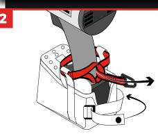
Secure the holster by pulling the strap tightly and clicking the closest button. Ensure the choke strap passes through the three choke guides by passing the D-Ring end through the loop end of the choke.
