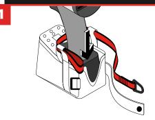
Insert the battery pack (whilst connected to the power tool) into the Battery Catch Holster XL..
