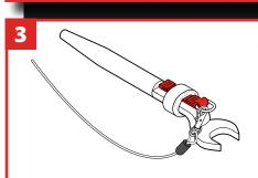
Your Tool Catch is now ready to be connected with a suitable GRIPPS® tether via the D-Ring.
