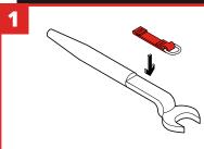
Place Tool Catch with metal ring facing away from the tools center of gravity, white tag facing up.
