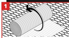
Place roll of GRIPPGrid on gridmesh floor in the desired location. Roll out the matting ensuring material is flat without kinks.
