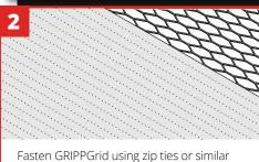
fasten GRIPPGrid using zip ties or similar fasteners in corners and along edging. Remove ties and roll back up for re-use when finished.
