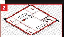
To secure the Modular Drop Mat, use cable ties to secure all of the eyelets to the workplace.
