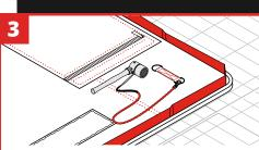
Ensure that tools are tethered to one of the 8 D-Ring anchor points on the Modular Drop Mat when working at height.
