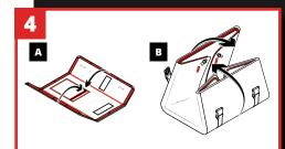
Once folded and secured, connect to the GRIPPS® Mule Bag using the carabiners and D-rings for easy transportation.
