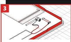
Ensure that tools are tethered to one of the 8 D-ring anchor points on the Modular Drop Mat when working at height.
