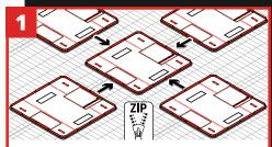
To connect multiple Modular Drop Mats together, align zips on both Modular Drop Mats and zip end-to-end.
