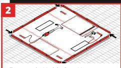
To secure the Modular Drop Mat, use cable ties to secure all the eyelets to the work surface.
