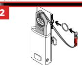
Thread tool ring back onto Retractor. The tool ring should be exposed outside of the holster.
