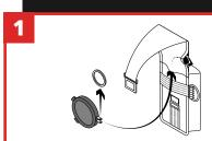
Remove tool ring form Retractor then insert Retractor into holster pocket. Feed end of Reactor cable out of holster pocket.
