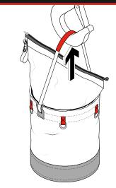
Only lift from the clearly identified load-rated lifting point on the strap of the bag. Ensure tools are tethered to the D-rings at all times. Do not lift from the carabiner.
