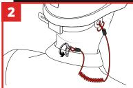
Push fabric all the way into the jaws of the clamp, ensuring that the clamp 'teeth' are totally covered by fabric.
