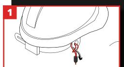
To connect to a hard hat, feed the looped end of the hard hat tether through an appropriate connector point on the hard hat.
