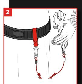
Attach tether to a desired anchor point such as holster D-Ring.
