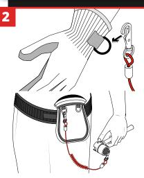
Attach tether to anchor point such as D-ring on a  ${\sf GRIPPS}^{\circledast}$  glove or bag.
