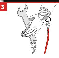
Once the tool ring is applied to your chosen tool, connect the tool ring to a GRIPPS® tether of choice.
