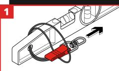
Feed the Swivel Catch through the pre-formed hole in the tool. Loop Swivel Catch back through itself. Your tool is now ready to be applied to a GRIPPS® Retractable Tool Belt via a GRIPPS® Retractor Unit.
