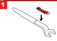
Place Tool Catch with metal ring facing away from the tools center of gravity, white tag facing up.
