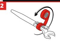
Wrap the tape around the tool 10x while stretching the tape to activate the selfvulcanizing feature, creating a secure connection. Ensure raised 'catch' is not covered by the tape. Pull on Tool Catch with force to test application.
