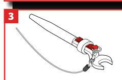
Your Tool Catch is now ready to be connected with a suitable GRIPPS® tether via the D-Ring.
