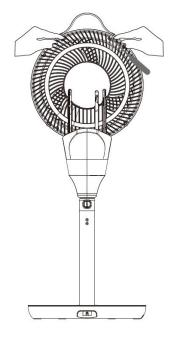
2. Squeeze the two tabs to the left and right of the screws and pull away. At the front of the fan blades there is a locking cap – unscrew the cap in a clockwise motion to remove the fan blades.
