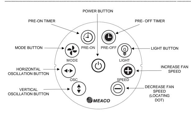
The following functions are only available via the remote control. All other buttons on the remote-control work in the same way as the control panel (see pages 5 and 6). The remote control has a range of approximately three metres. Before using the remote control, remove the plastic tab.
