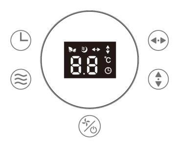
Please note all the buttons are touch sensitive and bleep when pressed. The buttons need to be pressed quickly, do not hold your finger on the button for longer than one second (unless when turning the air circulator ON/OFF, see below). Do not operate the controls on the base of the air circulator with your feet.
