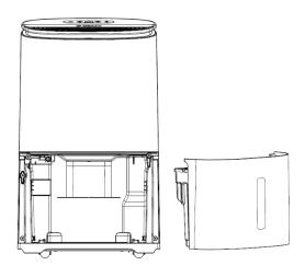
**Step 1:** Remove the water tank.
