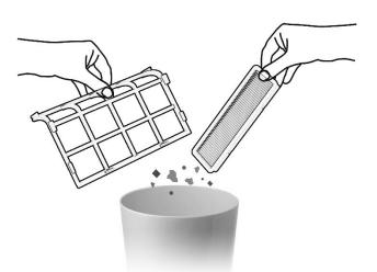
2. Rinse the filters if necessary. Do NOT rub the filters or use high-pressure water. Be sure to leave the filters to dry thoroughly before reinstalling them.
