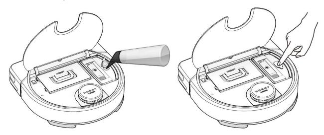
\*DO NOT use any other detergent or liquid to prevent blockage of the pipes and the spray nozzles.
