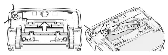
3. Use the cleaning tool to cut loose the tangled hair and debris to clean the brushroll, rinse then dry when needed.
