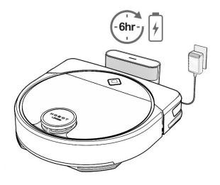
Plug power adapter into the charging station and place the flat end of the robot against the charging station.
