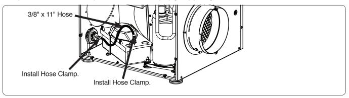
**Step 8:** Using Channel Locks, thread the other 3/8" Hose Barb Adapter into the Bulkhead Fitting on the exterior of the unit. Ensure the Adapter is threaded tightly, but do not over-tighten. Locate the 20' Hose contained in this kit. Insert one end of the Hose onto the 3/8" Hose Barb Adapter and secure using another Hose Clamp. Route Hose appropriately to Drain.
