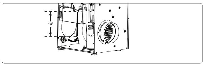
**Step 4:** Using Channel Locks, unthread the stock 5/8" Hose Barb Adapter out of the Bulkhead Fitting and set aside. Replace it with one of the 3/8" Hose Barb Adapters contained in the kit. Ensure the Adapter is threaded tightly, but do not over-tighten.
