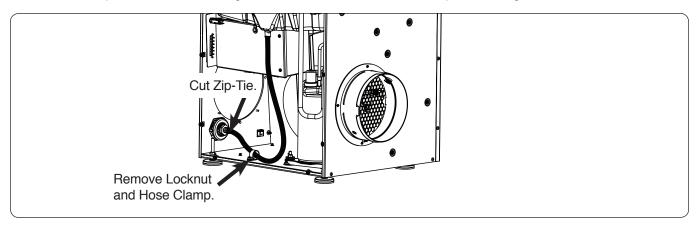
Step 3: Pull the Condensate Hose loose from the Fitting. Using Scissors or Side Cutters, cut the length of the Hose to 14" from the Drain Pan. Cut the end of the Hose at a 45 degree angle for proper drainage.
