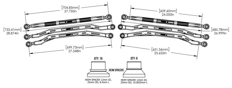
Use the (16) 8.4mm spacers for all of the inner/outer heim bearings Use the (8) 10mm spacers on the fixed inner mount points of the high clearance rods
