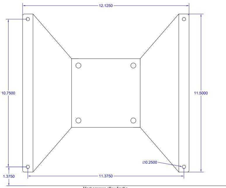
Most presses allow for the mount to be installed 1" from the edge of the bench.
