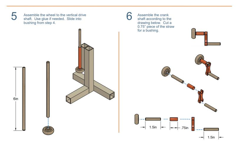
Carefully glue the crank shaft bushing onto the base lifting the vertical drive shaft in position. The crank arm should rotate freely.
