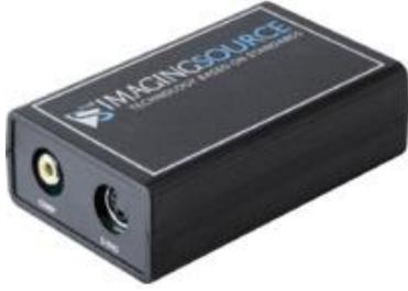
Even though digital machine vision cameras continue to grow in popularity, there are still an enormous number of analog video sources. Using a video-to-USB converter, analogue video sources become usable in a digital environment. The DFG/USB2pro converts analog video signals (PAL, NTSC, CCIR, EIA) into uncompressed image data streams, and supports digital and analog cameras in color and in monochrome. The model DFG/USB2aud additionally converts analogue audio signals.
