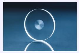
S-waveplate converts linear polarisation to radial or azimuthal polarisation and circular polarisation to an optical vortex.
