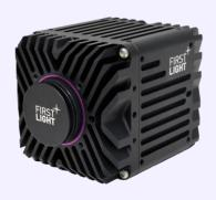
C-RED 2 Lite is the stabilised version of C-RED 2, able to run at 600 FPS with 32 electrons readout noise. To achieve this performance, C-RED 2 Lite integrates a 640 x 512 InGaAs PIN Photodiode detector with 15 µm pixel pitch for high resolution, which embeds an electronic shutter with integration pulses shorter than 5µs. The camera has no fan and is thermally stabilised, it can also be watercooled for better performance
