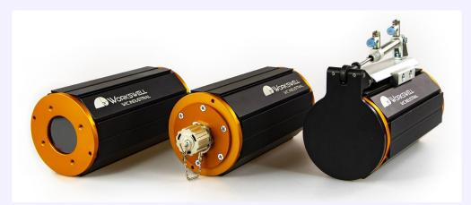
Designed and manufactured for easy and user-friendly plug & play integration for all process control and quality control applications. Customers can choose from two types of camera resolution, i.e. 640×512 or 336×256 pixels, and also from several different lenses. Temperature range can be chosen to 1,500 °C. 30mK sensitivity is offered as standard. Internal electronics are protected by a high IP66/IP67 rating enclosure and can be installed in harsh conditions from -50 °C to +200 °C.
