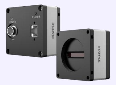
The iRAYPLE line scan camera provides resolutions from 2K,4K, 8K to 16K. Supports data interfaces GigE, Camera Link, 10GigE, and CXP-6, enabling efficient transmission of high-frequency data and suitable for fast-paced production lines. It supports various ISPs and algorithms, making it versatile for use in industries like PV, EV, display panels, and printing.
