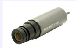
Fully adjustable bullet camera. 1/4" CMOS sensor with 480TVL and 0.3lx at F2.0 with M12 glass f3.8 F2.0.
