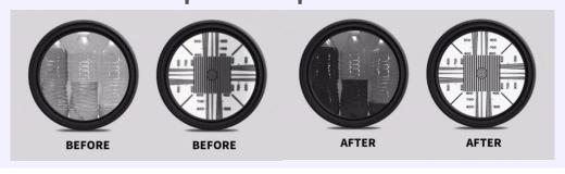
**Bandpass Filters** are one of the simplest ways to improve image quality. They have the unique ability to block unwanted ambient light while passing only the necessary light output – improving contrast and resolution.
